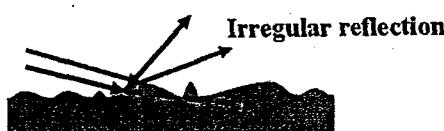
Figure 1: A schematic diagram showing a irregular reflection from the surface roughness.
