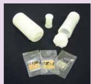
Capsules(back) and irradiation samples(front)
