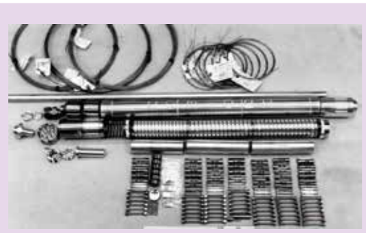
Irradiation capsules(back) and irradiation test pieces(front)
